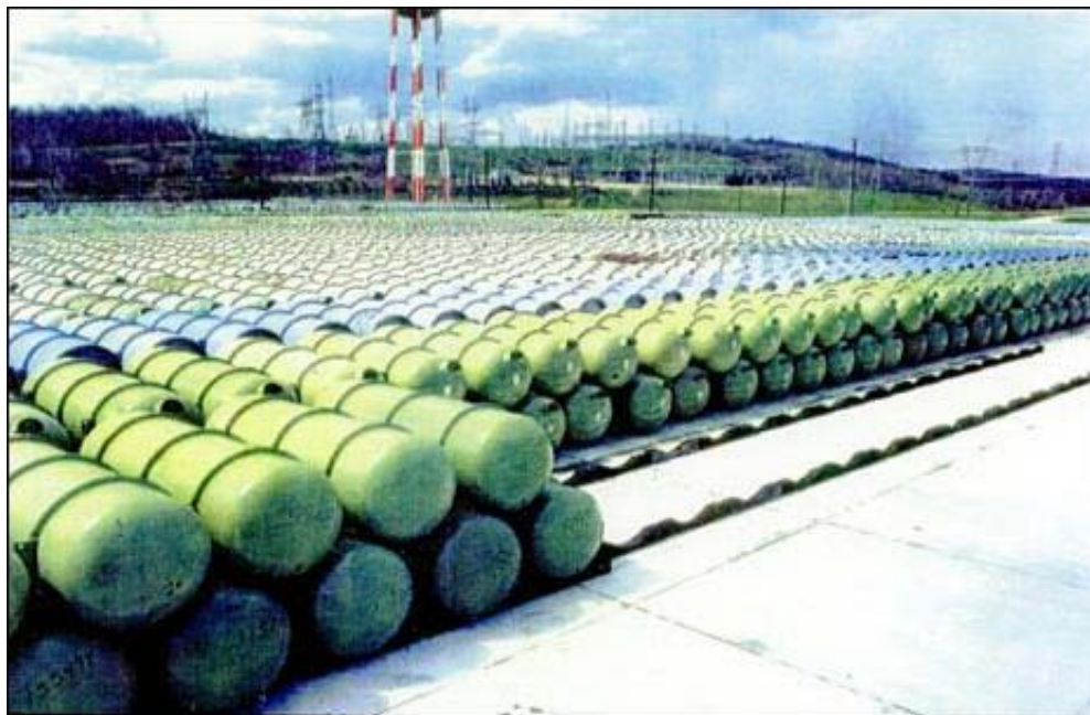
Figure 1. Accumulated \text{UF}_6 Cylinders at an Enrichment Plant Site
