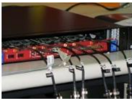
Fig. 6. CAEN V1720 waveform digitizer.
