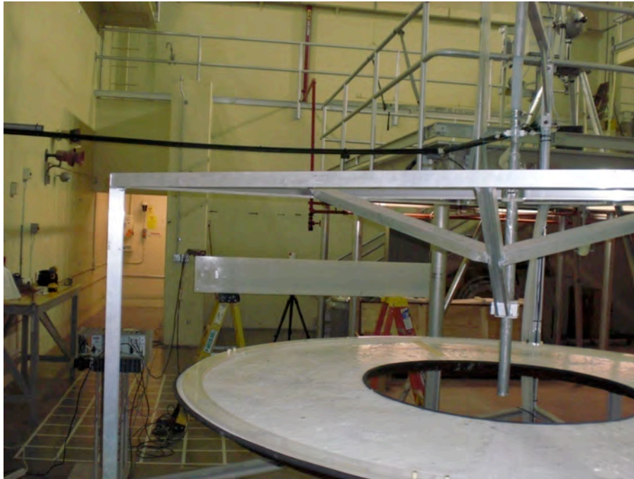
Figure 2: Boron-lined detector (in white, rectangular box resting on two ladders) being tested with gamma ray and neutron sources.
