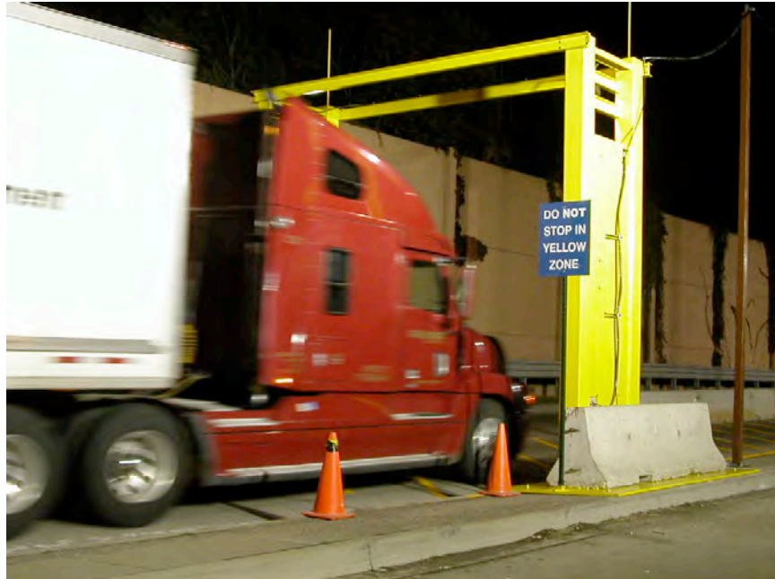
Figure 1. Typical RPM scanning a vehicle for radiological material. (Photo By D. Stromswold)
